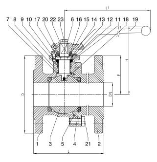
Flanged ball valve full bore face to face acc. to EN 558, GR.1 face to face acc. to EN 558, GR.27 flanges acc. to EN 1092 Specification:
