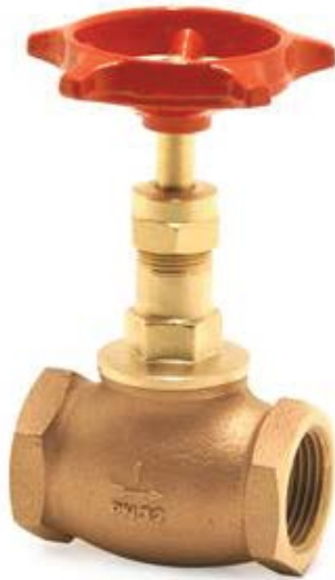
Bronze threaded globe valve with renewable non-metallic seat disk, female ends, PN32
