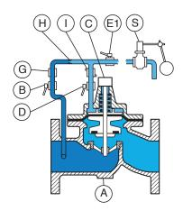
The level in the tank is low and the float switch S is fully open. The valve A is wide open and supplies the tank.
