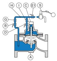
The float is in intermediary position, the float S switch is half closed. Consequently, the head loss increases the pressure in the upper chamber, the valve A will close. It will be completely closed as soon as no flow runs out from the float S switch in high position.
