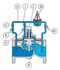
When the pilot M opens, pressure in the upper chamber is released and the valve A opens, reproducing the movement of the pilot.
