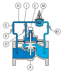
When the pilot M closes, pressure in the upper chamber rises also and forces the membrane to close the main valve A which reproduces the movement of the pilot.
