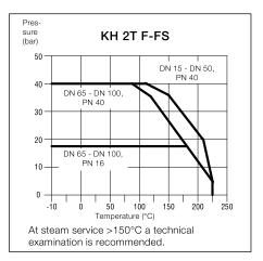
Ordering example: KH 2T F-FS, DN 65, PN 16, GR.1, 1.4408, safety spring locking device
