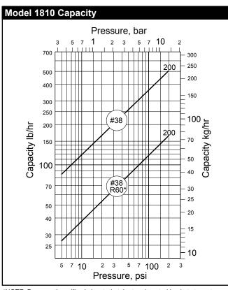
\*NOTE: Because the orifice is located at the top, inverted bucket steam traps handle dirt and scale better than other types of traps. However, in applications where extremely dirty conditions exist, care should be exercised in the use of all types of restricted-orifice, reduced-capacity traps.
